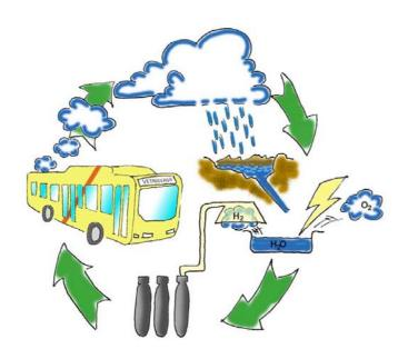
Iceland has the rare opportunity to operate a project, based on hydrogen fuel, in a next to zero CO<sub>2</sub> system. The hydrogen will be produced by electrolysis, where electricity is produced by geothermal steam turbines and hydropower.
